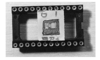
once the chip is visible, one can use microprobing needles or electron beam testers to access on-chip signals and extract data from the chip
